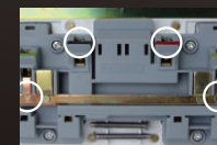
Double earth terminals for safer sockets
